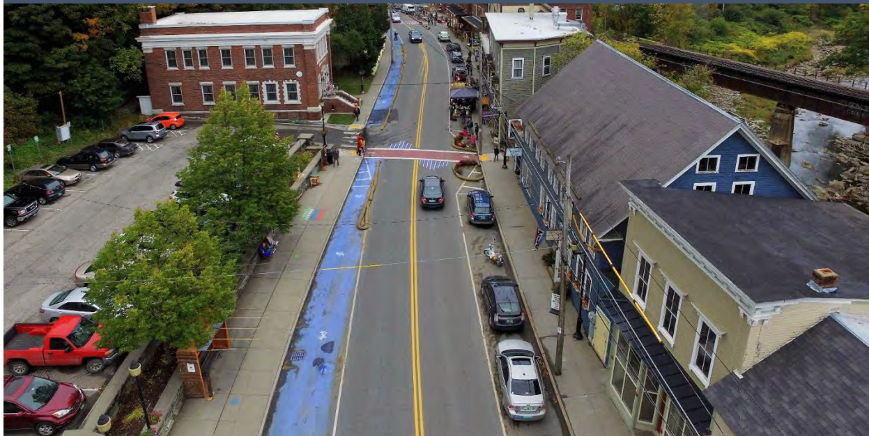
Figure 6. Demonstration shared use path and parklet along a Class 1 section of VT Route 12 in downtown Bethel, part of the Bethel Better Block initiative. To meet national standards this project would have needed to use a green paint, instead of blue, with no intermittent artwork, and added vertical delineation along the edge, in addition to the hay.
